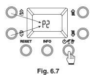
Pressing the mode button (  $\oplus \mathcal{T}^{\textcircled{B}}$ ) displays the parameter and by pressing the CH up and down buttons ( 1 ) you can adjust its value.
