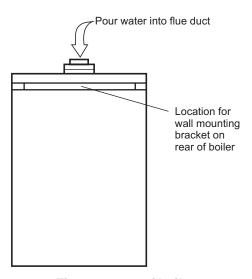
Fig. 4.3 - rear of boiler
