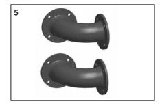
The flow and return headers are available in 2 dimensions, i.e. DN65 and DN100 and are connected to one another by the flange couplings, M12 or M16x55 bolts, spring washers and nuts. The low loss header and the complete installation can then be connected to it.
