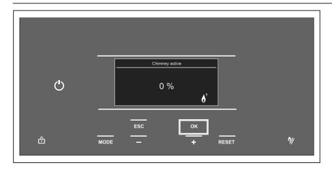
Step 2: O<sub>2</sub> / CO<sub>2</sub> check on low load
