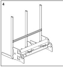
in the required location. When using several flow and return headers: connect the flow and return headers with the supplied gaskets, M12 (DN65) or M16 (DN100) bolts, spring washers and nuts. Align the flow and return header(s) horizontally using the adjustable 2. Place the gas line in its intended
