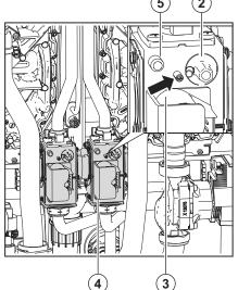
Step 3: Adjustment on the gas valve
