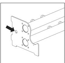
For condensate drainage, only corrosion-resistant and certified materials may be used. The drainage must be carried out in a frost-free space. The drainage pipe should have a slope, so as to avoid a backwash of the condensate.
