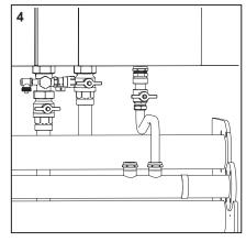
1-2. Keep the cap on the connections that are not used on the flow and return headers:
