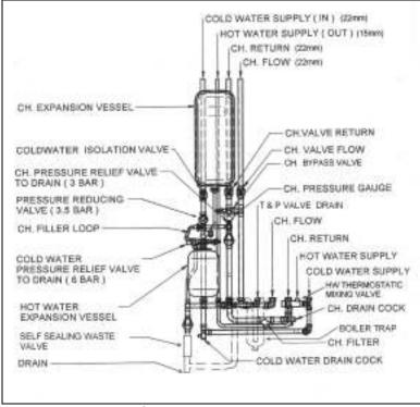
Pipework Assembly Components
