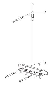
To mount the assembly bracket on a brick wall of sufficient thickness, use the screw plugs that are supplied. When you have determined the place of assembly, proceed as follows:
