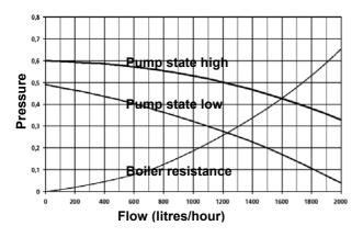
If set on automatic function the electronics switches the speed of the pump to "high" or "low", depending on the temperature demand:
