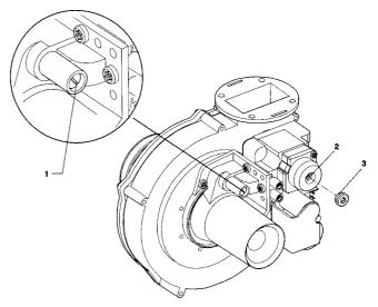
(1). Venturi screw – Full load adjustment
