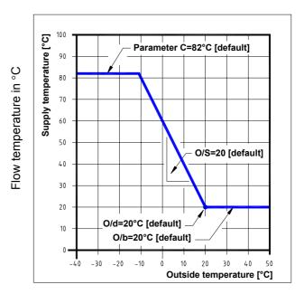
**O/b-value:** The setting of the minimal Heating flow temperature ( value in °C).
