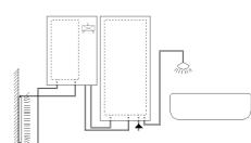
High efficiency boiler for central heating, suited for the connection of an external storage vessel for the indirect supply of tap water for shower and bath, etc.
