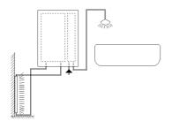
High efficiency Combi-boiler for central heating with a built-in tank (3 litres) for the supply of tap water for shower and bath, etc.
