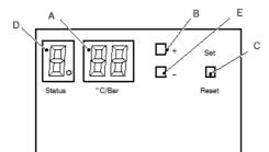
During operation, the display shows the status of the unit in the form of a code. To be able to read the codes, open the cover in front of the display. The display consists of three 7-segment LED's + three decimal points and three pushbuttons. The left 7-segment LED shows the status or the menu step.
