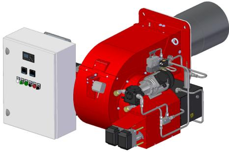
Burners for heavy oil at three stages, fan at high pressurisation, combustion head with adjustment at high efficiency and high flame stability complete of servomotors for the opening of the air shutters, suitable for heavy oil up to 20°C to 50°C and for BTZ heavy oil.
