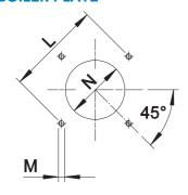
\* Suggested dimension of connection between burner and generator.
