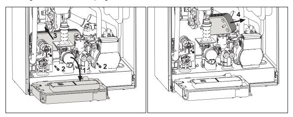
fig. 38- Plate to plate heat exchanger replacement/maintenance
