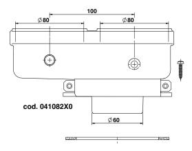
fig. 26- Twin flue appliance adaptor for separate ducts
