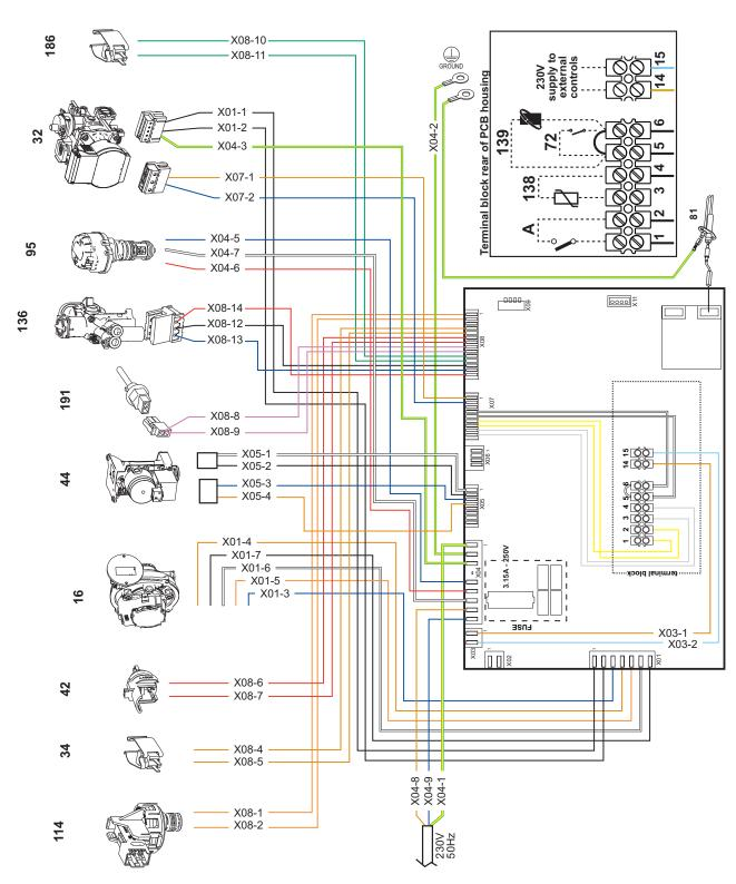
fig. 60- Wiring diagram
