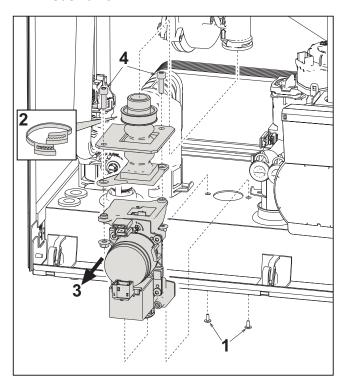
fig. 36- Gas valve replacement
