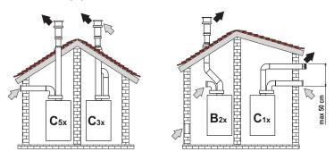
fig. 25- Examples of connection with Twin pipe system ( = Air / = Fumes)
