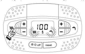
fig. 33- TEST mode (heating power = 100%)
