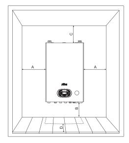
fig. 17 - Minimum distances around the boiler
