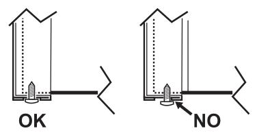
fig. 35 - Correct position of front panel
