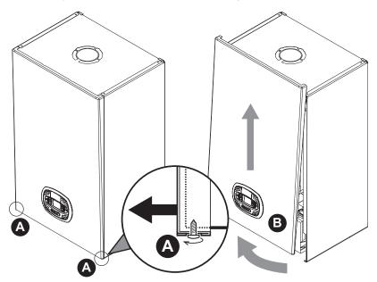
fig. 34- Front panel opening
