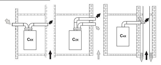
fig. 27- Examples of connection to collective flues ( = Air / = = Fumes)
