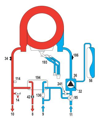
fig. 58- Hydraulic circuit
