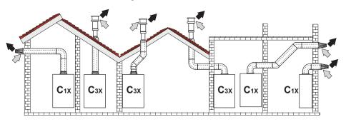
fig. 23 - Examples of connection with concentric chimney flues ( = Air / = = Fumes)
