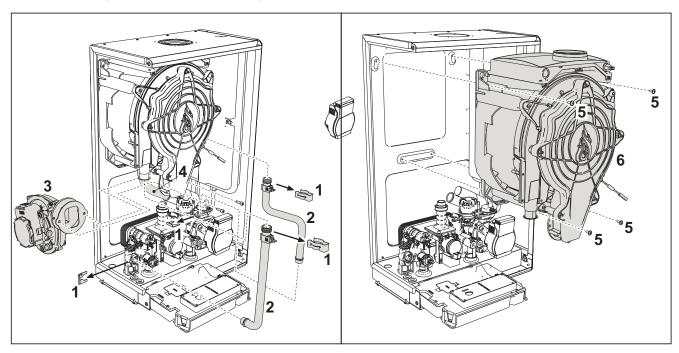
fig. 42- Main exchanger
