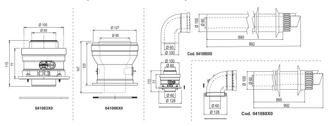
fig. 24- Appliance adaptors for concentric chimney flues
