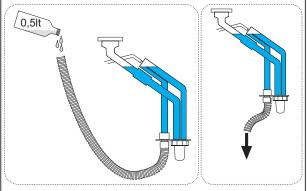
fig. 29- Condensate drain connection
