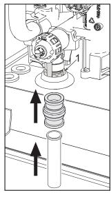
fig. 16- Safety valve with built in drain tap
