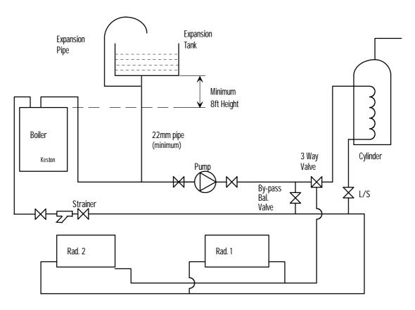
Figure 2.7.1: Open Vented System Diagram
