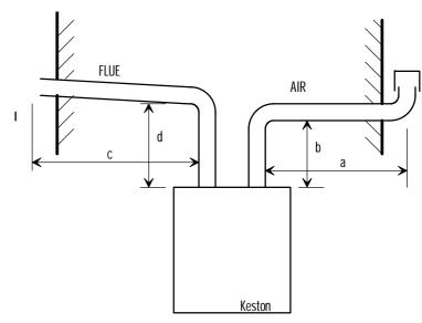
Figure 2.8.2 : Flue & Air Maximum Length Example
