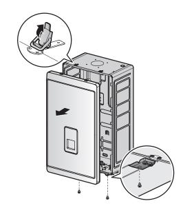
5. Once the front cover is removed, place it in a safe location to prevent accidental damage.
