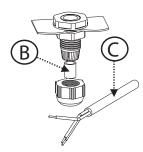
3. Insert cable "C" into the lid "A" together with the seal "B".
