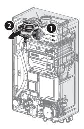
9. Remove the four bolts securing the chamber brackets.
