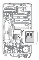
Figure 6. Set the DIP switches
