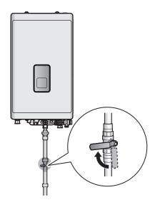
6. Close off any heating zones that do not require draining and open a purge valve to drain the central heating side. Open all domestic hot water taps completely to drain the water heating side. The water that remains in the plumbing lines will drain out.
