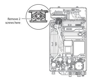
Figure 4. Access to Gas Orifice in Fan Assembly
