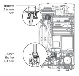
8. Remove the screw connecting the fan motor assembly and the mixing chamber, and then remove the fan motor assembly.
