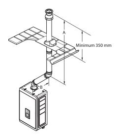
$\emptyset$ 60/100 => Max. length: A+B-(1 x 45°elbow) = 8-1 = 7 m  $\emptyset$ 80/125 => Max. length: A+B-(1 x 45°elbow) = 28-1 = 27 m
