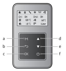
Menu button **Back button** b Access to the Main menu screen. Access to the previous screen. Up button **OK** button d Increases the temperature setting, Access to the selected item. parameter or moves up. Down button Power button Decreases the temperature setting, f e Turns the boiler on or off. parameter or moves down.
