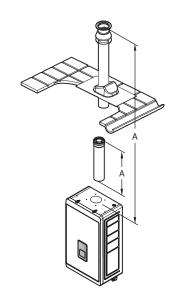
$\emptyset$ 60/100 => Max. length: A = 8 m  $\emptyset$ 80/125 => Max. length: A = 28 m
