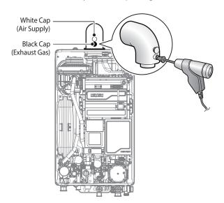
Figure 7. Insert the Analyser
