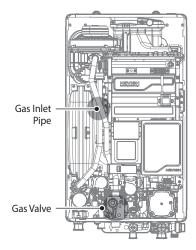
Figure 2. NCB500 Internal Components
