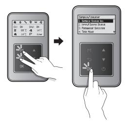
Press the Up button ( $\triangle$ ) or the Down button ( $\nabla$ ) to switch between the information items. Press the OK button ( $\bigcirc$ K) to select an item and view the information.
