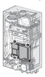
7. Remove the front panel assembly.
