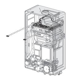
10. Remove the rubber packing at the top of the cover and put a Phillips screwdriver into the hole, and then loosen the middle bolt located at the back of the burner.
