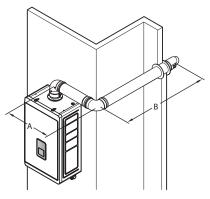
$\emptyset$ 60/100 => Max. length: A+B-(1 x 90°elbow) = 8-1.3 = 6.7 m  $\emptyset$ 80/125 => Max. length: A+B-(1 x 90°elbow) = 27-2.2 = 24.8 m
