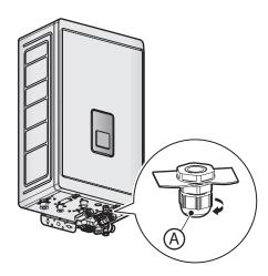
2. Remove the black silicon seal "B" from the cable gland and thread it onto cable "C".
