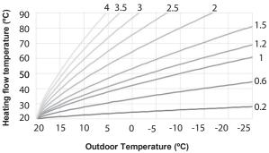
If there is an input from the outdoor temperature sensor, OTC (Outdoor Temperature Compensation) control will be enabled automatically. Also, if there is no input from the outdoor temperature sensor, OTC control will be disabled automatically.
