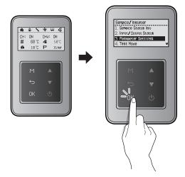
In the password screen, press the Up button ( $\blacktriangle$ ) or the Down button ( $\blacktriangledown$ ) to change numbers and places, and press the OK button (0K) to enter the password.
