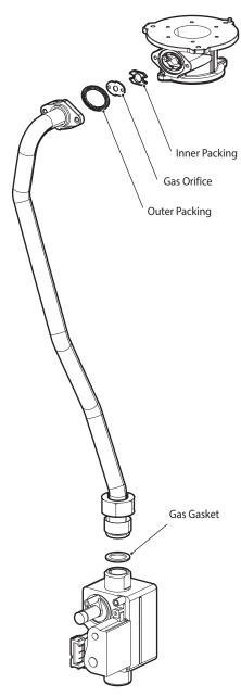
Figure 5. Exploded View of Gas Pipe Assembly (NCB500)
