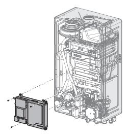
8. With the internal components exposed, locate the gas inlet pipe and the gas valve in the middle of the unit, as shown in Figure 2.
