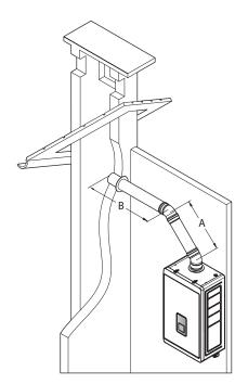
$\emptyset$ 60/100 => Max. length: A+B-(1 x 45°elbow) = 8-1 = 7 m  $\emptyset$ 80/125 => Max. length: A+B-(1 x 45°elbow) = 27-1 = 26 m
