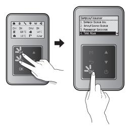
Press the Up button (  $\blacktriangle$  ) or the Down button (  $\blacktriangledown$  ) to switch between the test procedures. Press the OK button ( $\bigcirc$ K) to run a test procedure.
