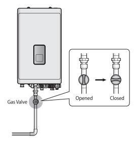
2. Open a hot water faucet. The boiler should turn on and the gas in the gas supply line will be purged.
