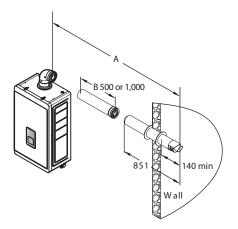
$\emptyset$ 60/100 => Max. length: A = 8 m  $\emptyset$ 80/125 => Max. length: A = 27 m
