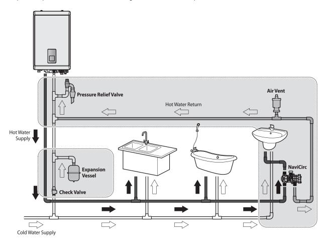
**Note** Refer to the following before installing the NaviCirc.
