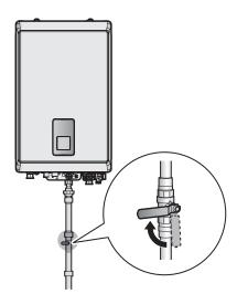
Close off any heating zones that do not require draining and open a purge valve to drain the central heating side. Open all domestic hot water taps completely to drain the water heating side. The water that remains in the plumbing lines will drain out.
