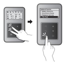
Press the Up button (  $\blacktriangle$  ) or the Down button (  $\blacktriangledown$  ) to switch between the test procedures. Press the OK button ( OK ) to run a test procedure.
