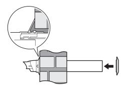
5. Although weather seals can be used, the flue must be installed that prevents lateral movement. The use of sand and cement to seal the flue to the fabric opening of the building would secure the flue as required. The seals can be put over the securing sand and cement as a decorative weather seals.
