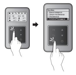
Press the Up button ( $\triangle$ ) or the Down button ( $\nabla$ ) to switch between the list items or to increase/decrease setting values. Press the OK button ( $\bigcirc$ K) to select an item or to confirm after making changes.
