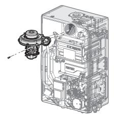
9. Remove the five bolts securing the chamber brackets.
