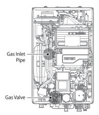
Figure 2-2. NCB700-3S/54K Internal Components
