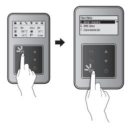
A list of 10 recent errors are displayed on the screen, with the most recent error displayed at the top of the list.
