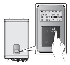
3. Press the OK button (○K) to select the DHW temperature (♠). The highlighted section will flash.
