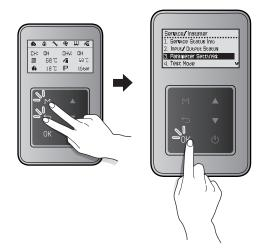
In the password screen, press the Up button ( $\blacktriangle$ ) or the Down button ( $\blacktriangledown$ ) to change numbers and places, and press the OK button ( $\bigcirc$ K) to enter the password.
