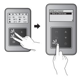
Press the Up button (  $\blacktriangle$  ) or the Down button (  $\blacktriangledown$  ) to switch between the operation modes. Press the OK button (0K) to select an operation mode.
