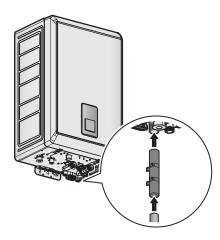
The drain line can be connected to the condensate trap using a condensate trap hose. The hose connection must be secured with a hose clip.
