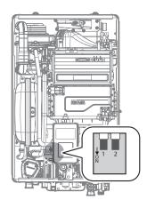
Figure 6. Set the DIP switches
