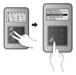
Press the Up button ( $\triangle$ ) or the Down button ( $\nabla$ ) to switch between the information items. Press the OK button ( $\bigcirc$ K) to select an item and view the information.
