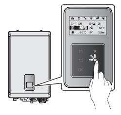
2. Press the OK button (○K) to select the central heating temperature (III). The highlighted section will flash.
