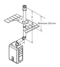
$\emptyset$ 60/100 => Max. length: A+B-(1 x 45°elbow) = 21-1.2=19.8 m  $\emptyset$ 80/125 => Max. length: A+B-(1 x 45°elbow) = 70-1.2=68.8 m
