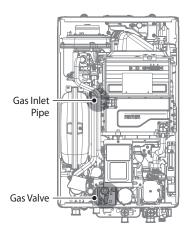
Figure 2-1. NCB700-2S+/42K Internal Components
