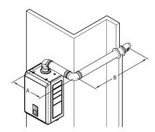
$\emptyset$ 60/100 => Max. length: A+B-(1 x 90°elbow) = 20-2.4=17.6 m  $\emptyset$ 80/125 => Max. length: A+B-(1 x 90°elbow) = 68-2.4=65.6 m
