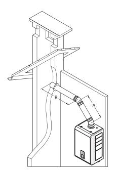
$\emptyset$ 60/100 => Max. length: A+B-(1 x 45°elbow) = 20-1.2=18.8 m  $\emptyset$ 80/125 => Max. length: A+B-(1 x 45°elbow) = 68-1.2=66.8 m
