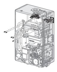
10. Remove the two screws connecting the ignition transformer to the heat exchanger and then remove the ignition transformer.
