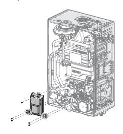
**Note** When removing the front panel, label all wires and make sure all wires are disconnected.
