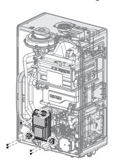
7. Remove the front panel assembly.
