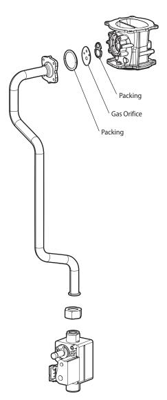
Figure 5-1. Exploded View of Gas Pipe Assembly (NCB700-2S+/42K)
