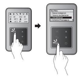
Press the Up button ( $\blacktriangle$ ) or the Down button ( $\blacktriangledown$ ) to switch between the list items or to increase/decrease setting values. Press the OK button ( $\bigcirc$ K) to select an item or to confirm after making changes.
