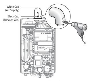
Figure 7. Insert the Analyser
