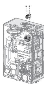
11. Remove the rubber packing at the top of the cover and put a Phillips screwdriver into the hole, and then loosen the middle bolt located at the back of the burner.
