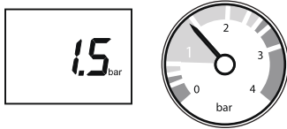
Fig.47 Restore water pressure
