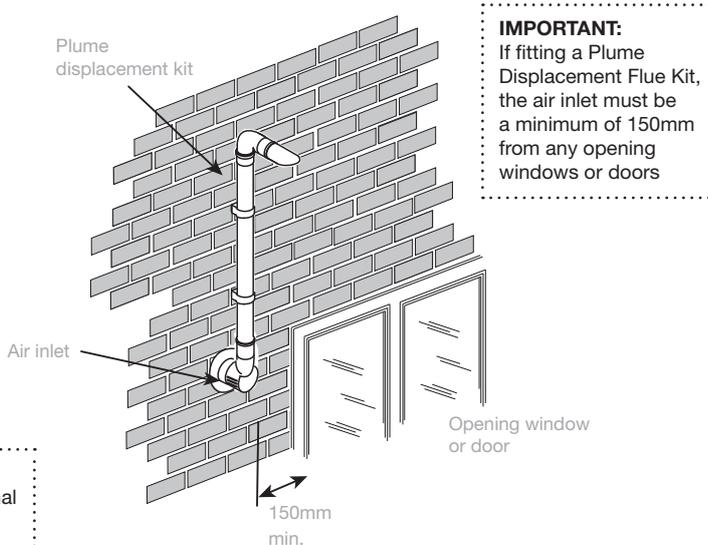
\*This can be reduced to 25mm by using item 6/7/8 flue deflector.
