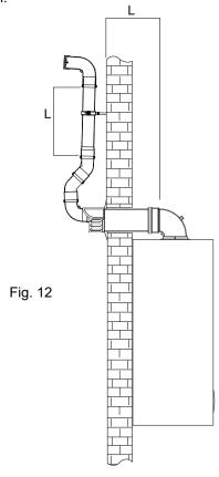
L+L max 6000 mm minimum plume kit length 500 mm
