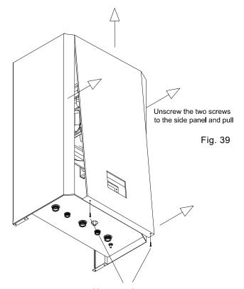
Unscrew the screws pull forward and lift up
