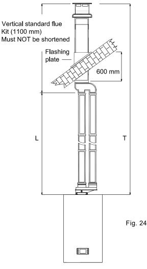
Straight flue L= 42 m max + terminal T= Max length 43 m
