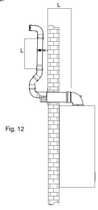
L+L max 6000 mm minimum plume kit length 500 mm
