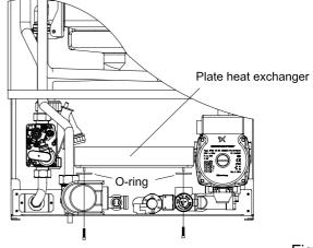
Unscrew the two allen screws and lift up the plate heat exchanger
