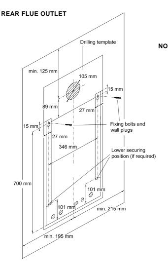
NOTE: The position of the appliance must provide minimum side clearances of 5mm as the side panels do not require removing for servicing. However, if the option is preferred to remove the panels then a minimum clearance of 55mm is required.
