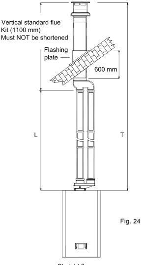
Straight flue L= 42 m max + terminal T= Max length 43 m
