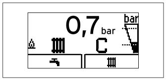
7.2 Display of the filling pressure for the heating system is too
