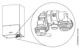
Fig. 7 Integral filling link location
