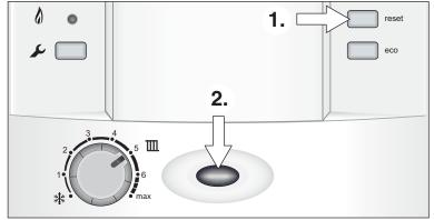
Fig. 5 Reset button and mains light
