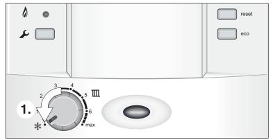
Fig. 3 Switch off central heating
