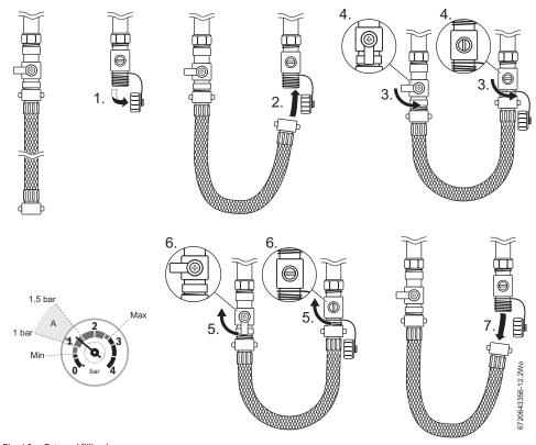
Fig. 10 External filling loop
