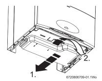
Fig. 6 Remove the bottom panel
