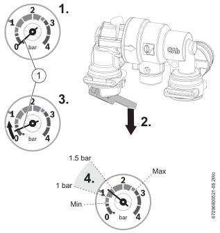
Fig. 8 Keyless filling link
