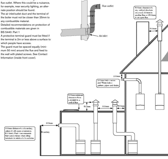
Deductions metre off the total flue length for every 45° bend used. Deduct two metres off the total flue length for every 90° band used 1000mm The flue turnst has a built-in angle of 3" to 1000enen ensure that the condensate flows back to the boiler for eafs disposal via the condensate waste pipe.
