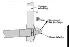
The flue cannot be lower than 1000mm from the top of a light well due to the build up of combustion products
