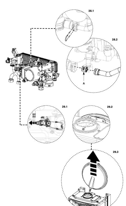
**NOTE:** Remove the Hydraulic block from the boiler (Refer to page 51).
