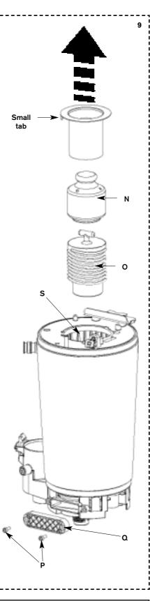
IMPORTANT: IF THE JOINT BETWEEN THE AIR/GAS MANIFOLD AND THE HEAT EXCHANGER IS DISTURBED THE SEALING GASKET MUST BE REPLACED.
