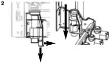
3. Hang the boiler on to the wall mounting frame by the two brackets positioned left and right at the top rear of the appliance. Do not lift the appliance by the air gas manifold. There are two handling holes incorporated into the inner casing left and right in the lower section of the appliance.
