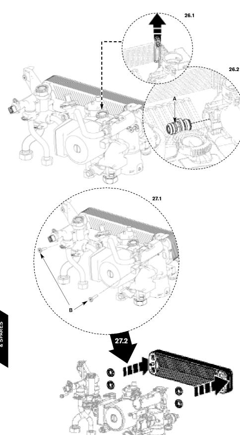
NOTE: Remove the Hydraulic block from the boiler (See removing the Hydraulic Block on page 51).
