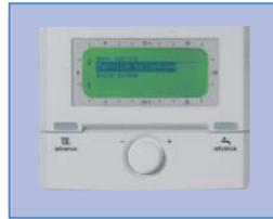
A seven day programmer with easy-to-use text display with automatic time and date setup, automatic summer/winter time changeover and a backlight for use in low light conditions. Three on/off periods can be set per day. The TD200 can be fascia mounted or hard wired outside the boiler using
