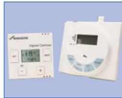
A seven day digital programmable RF thermostat with a seven day programmer/receiver in the boiler fascia. The transmitter is the tried and tested Optimiser as available with other Worcester boilers. The optimum start feature, where the thermostat delays the firing of the boiler until necessary, is a useful energy-saving option.
