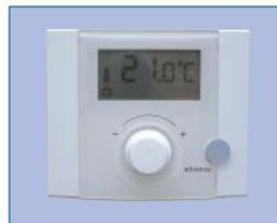
A hard wired optimising room temperature controller with digital display for use with the TD200. The display shows current and desired temperature and an advance button allows the user to move to the next heating switch point on the TD200.
