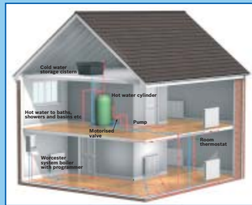
System boiler layout
