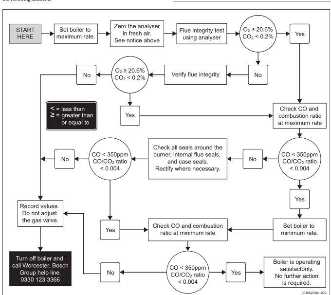
Fig. 66 Commissioning checks flow chart
