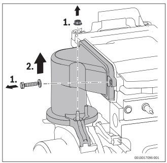
Fig. 76 Removing the air-gas manifold
