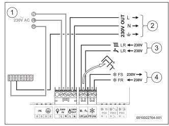
Fig. 57 External controls connections example
