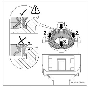
Fig. 90 Pressing on the gasket
