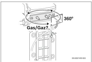
Fig. 87 Checking for leaks with an inspection mirror. Observe for misting.
