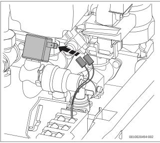
Connecting the automatic filling facility Fig. 54
