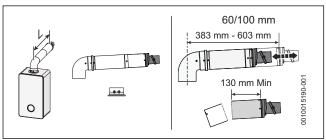
Fig. 12 Horizontal flue option
