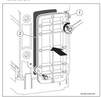
Fig. 85 Re-fitting the access cover
