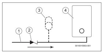
Fig. 9 Mini expansion vessel location
