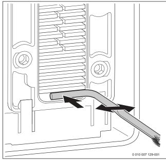
Fig. 84 Cleaning debris
