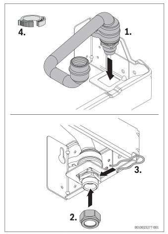
Fig. 42 Connect PRV discharge pipe
