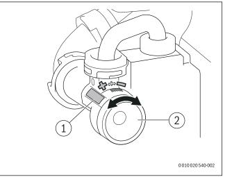
Fig. 93 Setting the adjustable venturi
