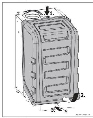
Fig. 63 Refit combustion casing
