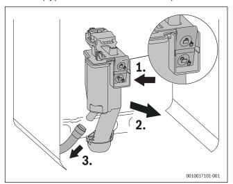
Fig. 88 Removing the condensate trap
