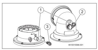
Fig. 67 Flue integrity check test point
