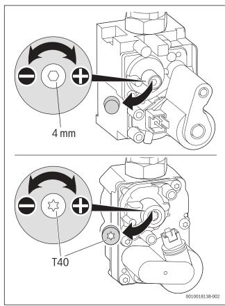
Fig. 95 Setting the CO<sub>2</sub> content (above: SIT valve, below: Honeywell valve)
