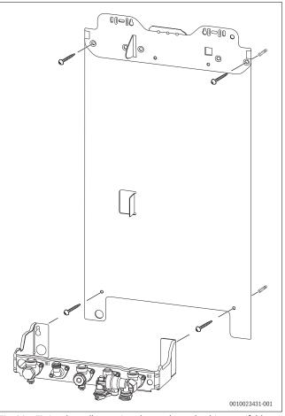
Fig. 39 Fitting the wall mounting plate and pre-plumbing manifold
