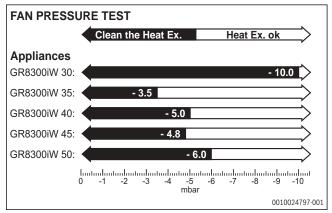
Fig. 73 Fan pressure test values
