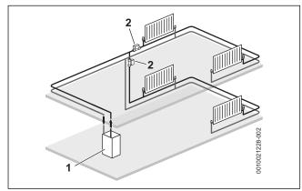
Fig. 7 Separated heating zones
