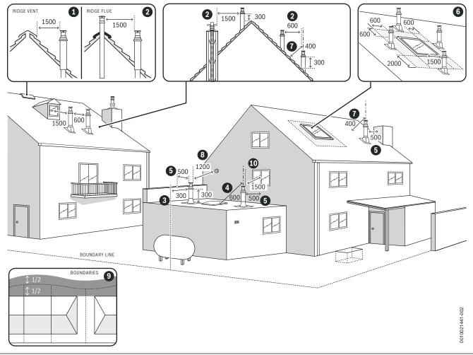
Fig. 26 Vertical flue terminal positions
