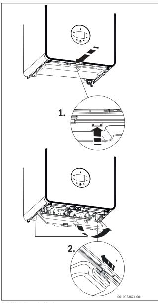
Fig. 70 Removing bottom panel
