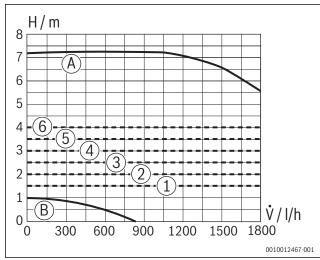
Fig. 105 Pump characteristic maps and pump curves
