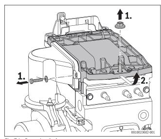
Fig. 74 Removing the burner cover
