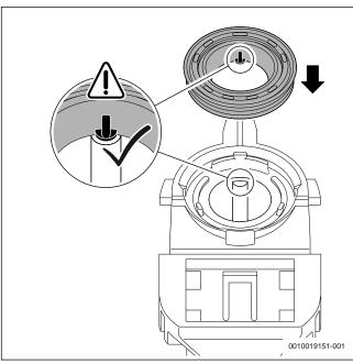
Fig. 89 Aligning the new gasket with the condensate trap
