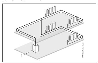
Fig. 6 Single central heating circuit example
