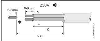
Fig. 55 Mains voltage (power cables) preparation
