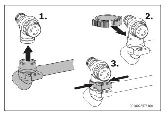
Fig. 44 Fitting the pipe on the (heating) pressure relief valve
