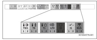
Fig. 53 Low voltage (signal cables) terminal strip
