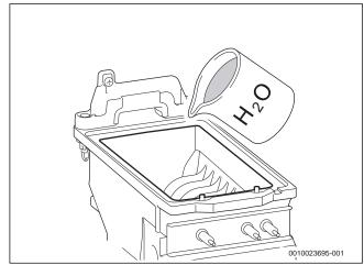
Fig. 83 Pour water into the heat exchanger
