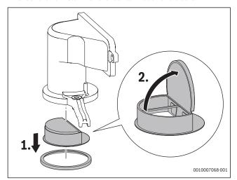
Fig. 77 Non-return valve in the air-gas manifold
