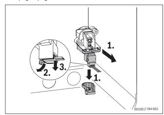
Fig. 102 Removing the motor of the 3-way valve
