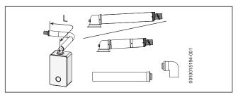
Fig. 16 Horizontal flue option
