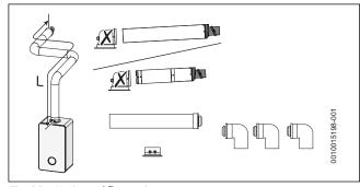
Fig. 20 Horizontal flue option
