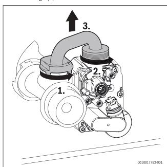
Fig. 97 Removing the gas pipe
