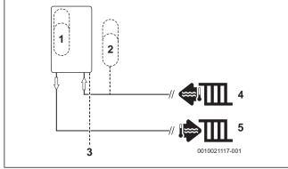
Fig. 4 Additional expansion vessel
