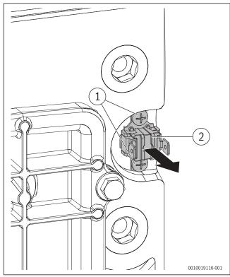
Fig. 96 Removing overheat thermostat
