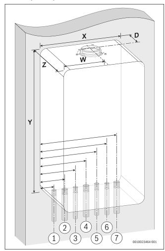
Fig. 2 Pipe and flue outlet dimensions
