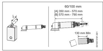
Fig. 13 Horizontal flue option
