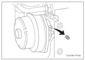
Fig. 72 Fan pressure test point
