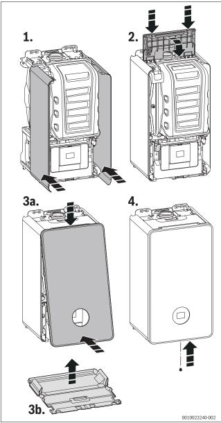
Fig. 69 Fitting the appliance casing
