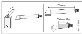
Fig. 14 Horizontal flue option
