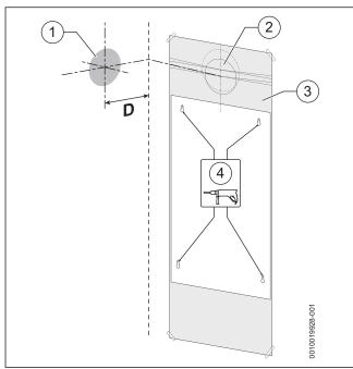
Fig. 37 Wall mounting template
