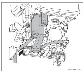
Fig. 46 Condensate connection
