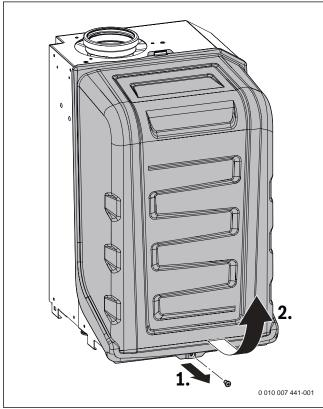
Fig. 92 Removing the combustion cover
