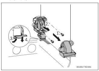
Fig. 103 Removing the 3-way valve
