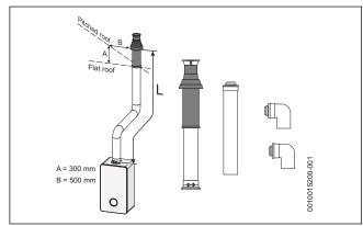
Fig. 22 Vertical flue option
