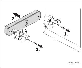
Fig. 104 Removing the plate heat exchanger
