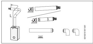
Fig. 19 Horizontal flue option
