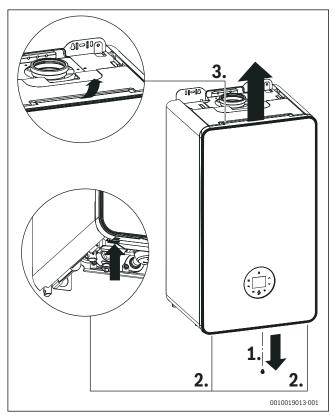
Fig. 71 Removing outer case
