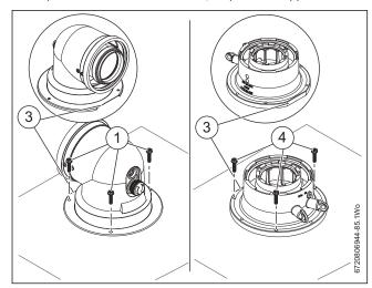
Fig. 49 Flue turret/adaptor connection
