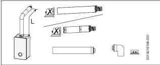
Fig. 18 Horizontal flue option
