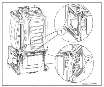
Fig. 38 Transport, lifting and handling
