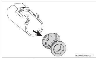
Fig. 101 Removing the flow turbine at the cold water pipe
