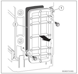
Fig. 80 Access cover removal
