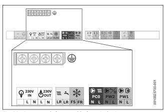
Fig. 52 Power supply (power cables) terminal strip
