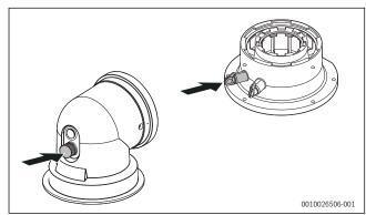
Fig. 94 Flue gas test point
