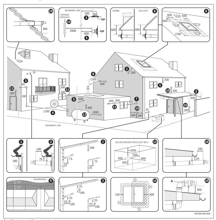
Fig. 27 Horizontal flue terminal positions
