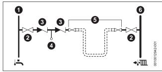
Fig. 8 External filling loop system fill example
