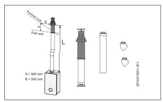
Fig. 23 Vertical flue option
