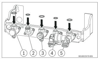
Fig. 41 Fitting the sealing washers
