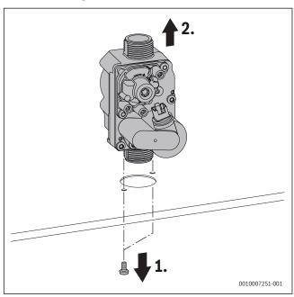
Fig. 99 Removing the gas control valve
