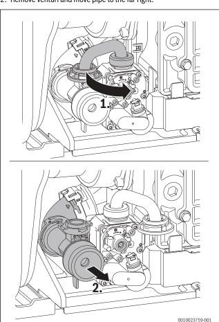
Fig. 78 Venturi removal
