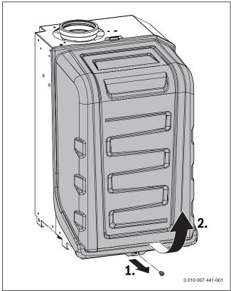
Fig. 61 Removing the combustion cover
