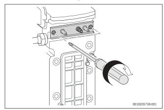
Fig. 86 Installing electrode set
