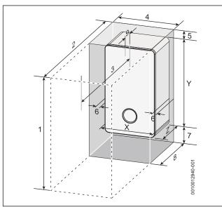
Fig. 11 Appliance minimum clearances
