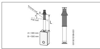
Fig. 21 Vertical flue option
