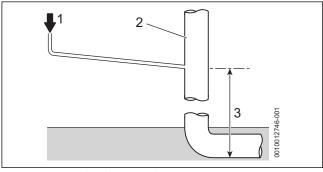
Fig. 29 Disposal to soil vent stack
