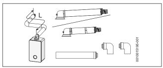
Fig. 17 Horizontal flue option
