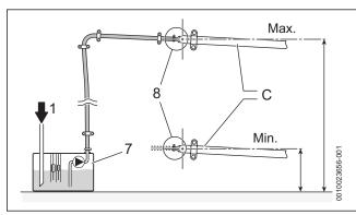
Fig. 31 Condensate pump example
