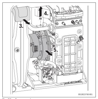
Fig. 79 Fan removal
