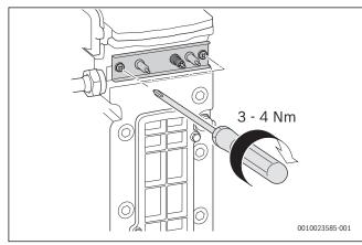
Fig. 88 Installing electrode set
