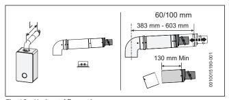
Fig. 12 Horizontal flue option
