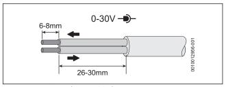
Fig. 57 Low voltage (signal cables) preparation
