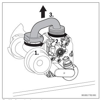
Fig. 99 Removing the gas pipe
