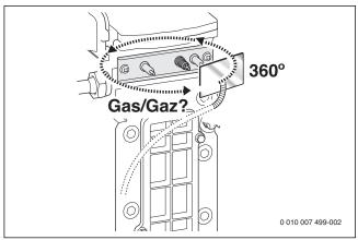
Fig. 89 Checking for leaks
