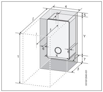
Fig. 11 Appliance minimum clearances
