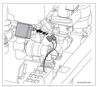
Fig. 55 Connecting the automatic filling facility
