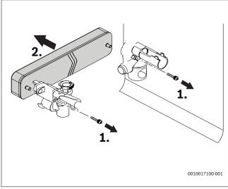
Fig. 106 Removing the plate heat exchanger
