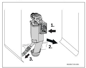
Fig. 90 Removing the condensate trap
