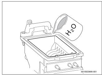
Fig. 85 Pour water into the heat exchanger
