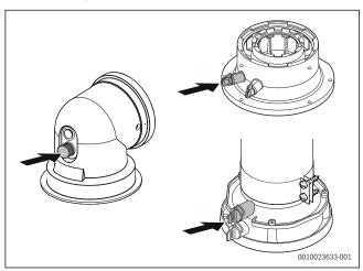
Fig. 96 Flue gas test port
