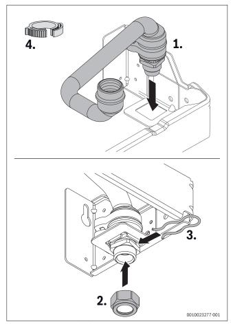
Fig. 43 Connect PRV discharge pipe
