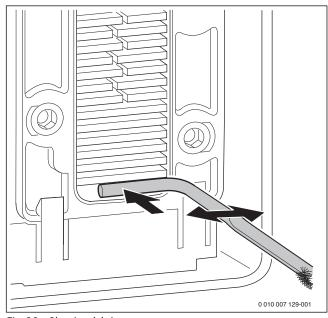
Fig. 86 Cleaning debris
