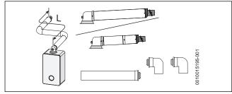
Fig. 17 Horizontal flue option
