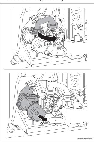
Fig. 80 Venturi removal
