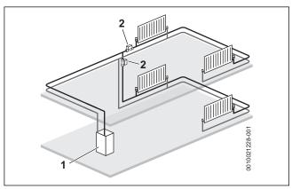
Fig. 7 Separated heating zones
