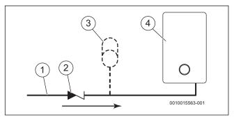
Fig. 9 Mini expansion vessel location
