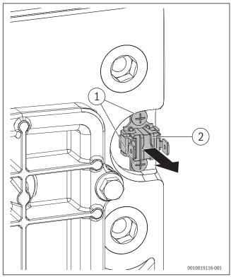
Fig. 98 Removing overheat thermostat
