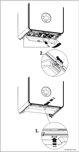
Fig. 72 Removing bottom panel
