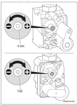
Fig. 97 Setting the CO<sub>2</sub> or O<sub>2</sub> content (above: SIT valve, below: Honeywell valve)
