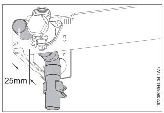
Fig. 46 Fitting the condensate pipes to the mounting plate
