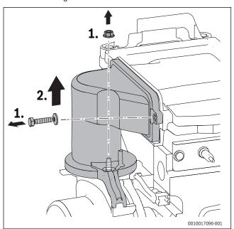
Fig. 78 Removing the air-gas manifold
