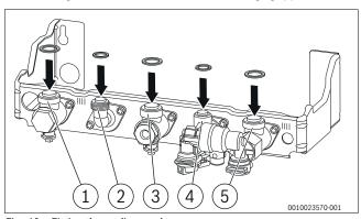
Fig. 42 Fitting the sealing washers
