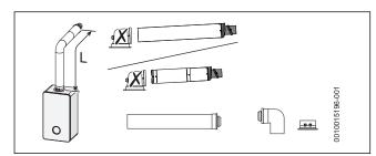
Fig. 18 Horizontal flue option
