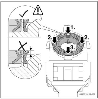
Fig. 92 Pressing on the gasket
