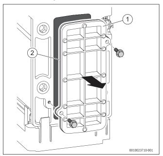
Fig. 82 Access cover removal
