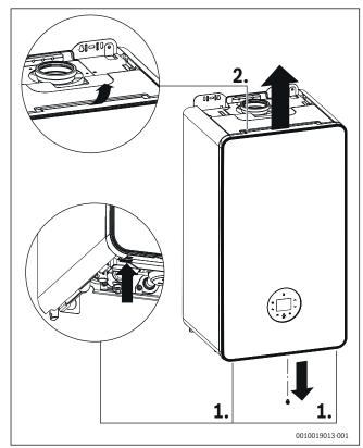
Fig. 73 Removing outer case
