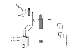
Fig. 22 Vertical flue option
