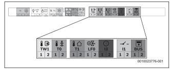
Fig. 54 Low voltage (signal cables) terminal strip
