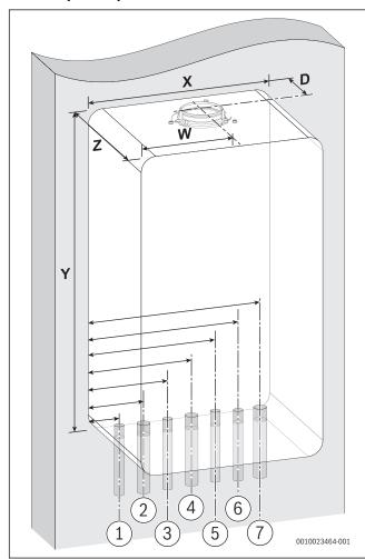
Fig. 2 Pipe and flue outlet dimensions
