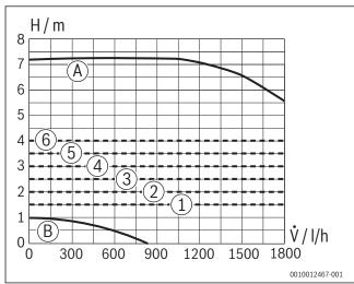
Fig. 107 Pump characteristic maps and pump curves
