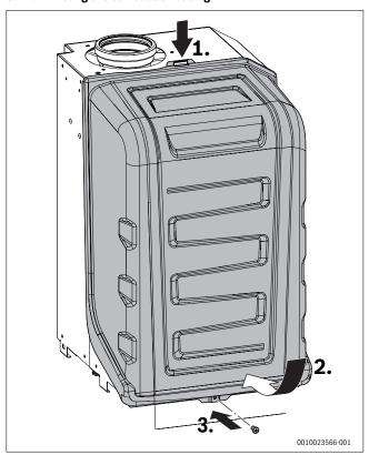
Fig. 70 Fitting the combustion casing
