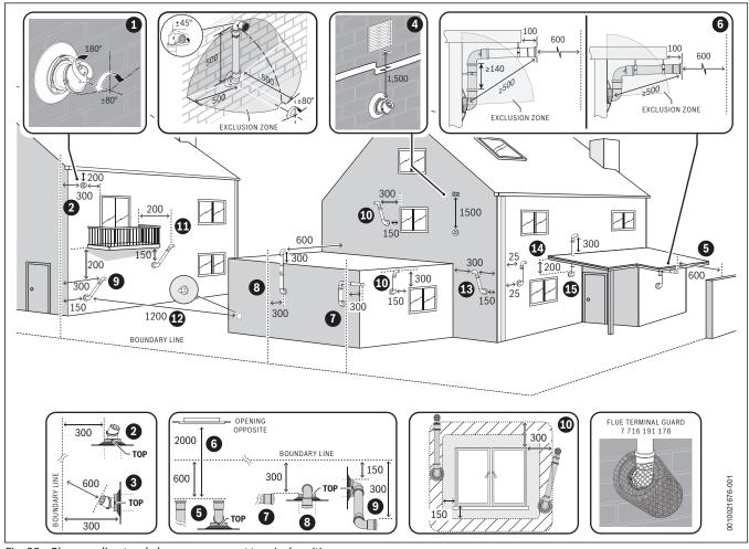
Fig. 28 Plume re-direct and plume management terminal positions
