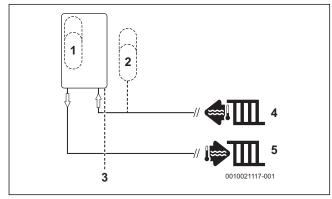
Fig. 4 Additional expansion vessel
