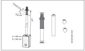
Fig. 23 Vertical flue option
