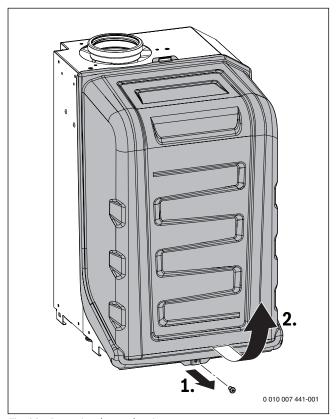
Fig. 62 Removing the combustion cover
