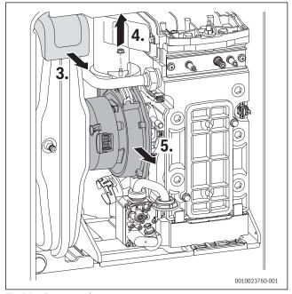
Fig. 81 Fan removal
