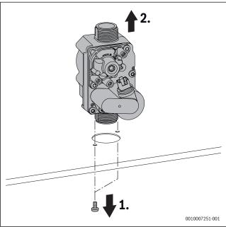
Fig. 101 Removing the gas control valve
