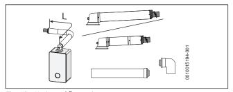
Fig. 16 Horizontal flue option
