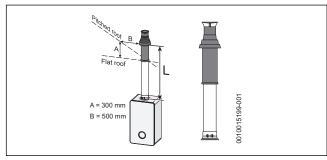
Fig. 21 Vertical flue option
