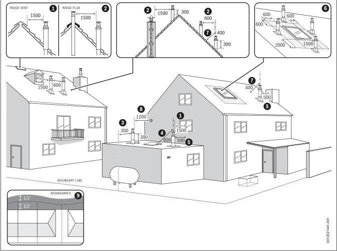
Fig. 26 Vertical flue terminal positions
