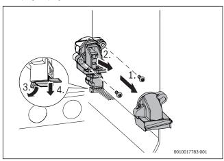
Fig. 105 Removing the 3-way valve
