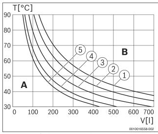
Fig. 5 Curves for the expansion vessel
