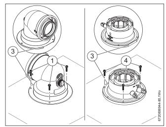
Fig. 50 Flue turret/adaptor connection
