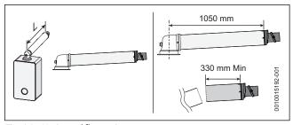
Fig. 14 Horizontal flue option
