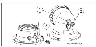
Fig. 68 Flue integrity check test point
