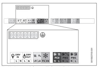
Fig. 53 Power supply (power cables) terminal strip
