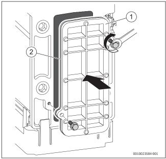
Fig. 87 Re-fitting the access cover
