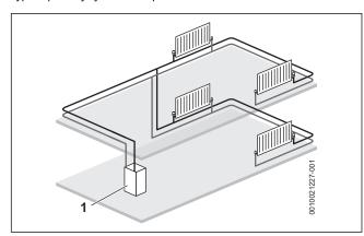
Fig. 6 Single central heating circuit example
