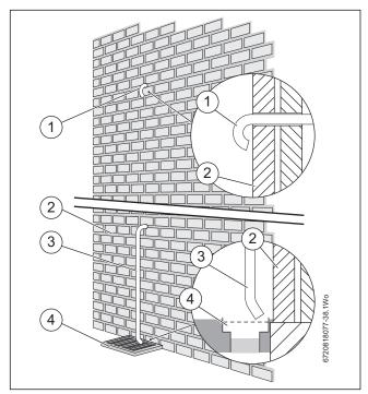
Fig. 36 Pressure relief pipe work
