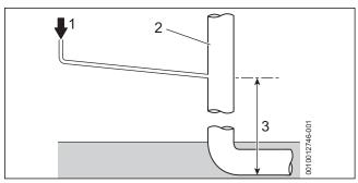
Fig. 29 Disposal to soil vent stack
