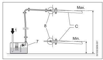
Fig. 31 Condensate pump example
