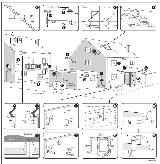
Fig. 27 Horizontal flue terminal positions
