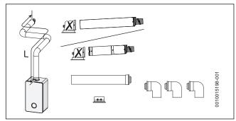
Fig. 20 Horizontal flue option
