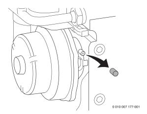
Fig. 74 Fan pressure test point
