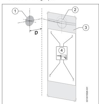
Fig. 38 Wall mounting template
