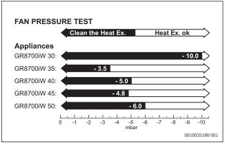
Fig. 75 Fan pressure test values
