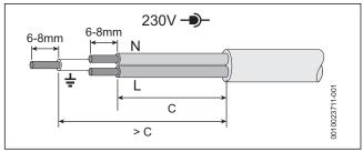
Fig. 56 Mains voltage (power cables) preparation
