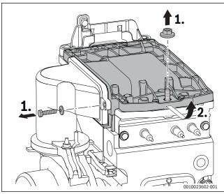
Fig. 76 Removing the burner cover
