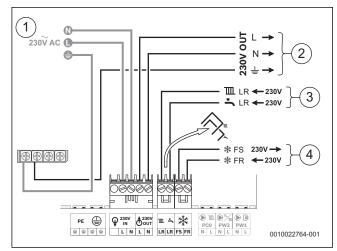
Fig. 58 External controls connections example
