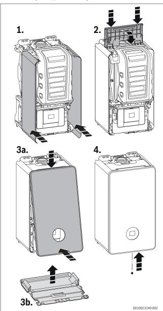
Fig. 71 Fitting the appliance casing
