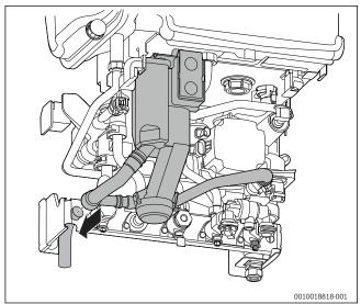
Fig. 47 Condensate connection
