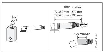
Fig. 13 Horizontal flue option
