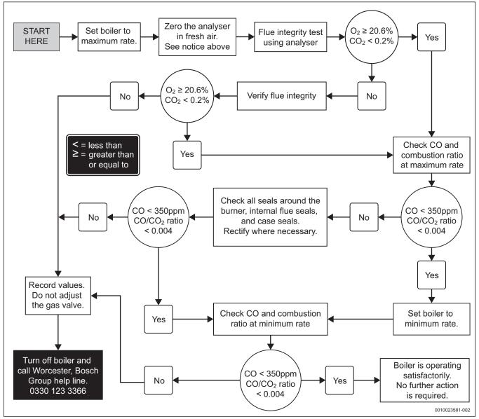
Fig. 67 Commissioning checks flow chart
