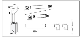
Fig. 19 Horizontal flue option
