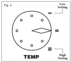
The control knob has a range of adjustment as indicated by the symbols.
