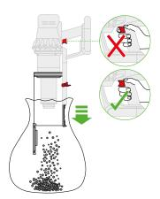
To release the dirt: Hold the machine over the bin in a downwards position.
