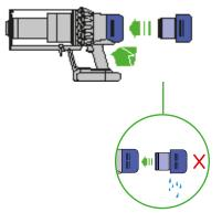
Remove the filter unit by twisting it anti-clockwise. Gently pull it away from the machine.
