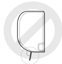
• Setting the louver at too small an angle when using COOL or HEAT mode, can reduce the performance of the AC due to restricted air flow.
