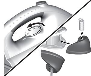
6. Turn the **temperature dial** back to its minimum setting. Then, turn off the steam generator iron and disconnect it from the mains supply. **Empty the water tank** and allow the iron to cool completely prior to storage.
