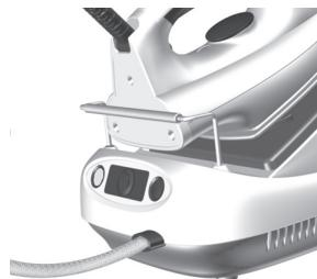
2. **When the power switch is pressed,** the power lamp will light. Wait for one to two minutes, until the steam lamp lights.
