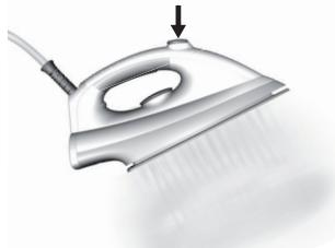
3. **To activate the steam,** press the steam button. When releasing the button, use up the steam before putting it back on the iron rest of the steam station.
