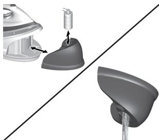
**4. Always allow the iron to cool fully on the iron rest before stowing away. Once the iron is cool, empty the water tank. Store the steam generator iron.**
