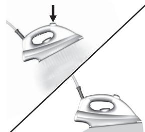
**9. When the steam lamp lights, press and hold the steam button for about one minute to get steam, then hold one more minute in order to clean the steam generating system.**
