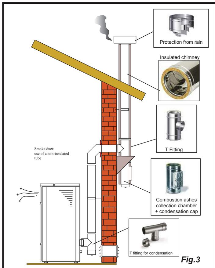
It is possible to use an existing chimney or a shaft via ducting. For this type of installation the standards on ducted smoke evacuation systems must be complied with. In the lower part of the chimney pot, inside the home, there is a "T" type fitting installed; externally there is another one installed, so that the outside section can be inspected.
