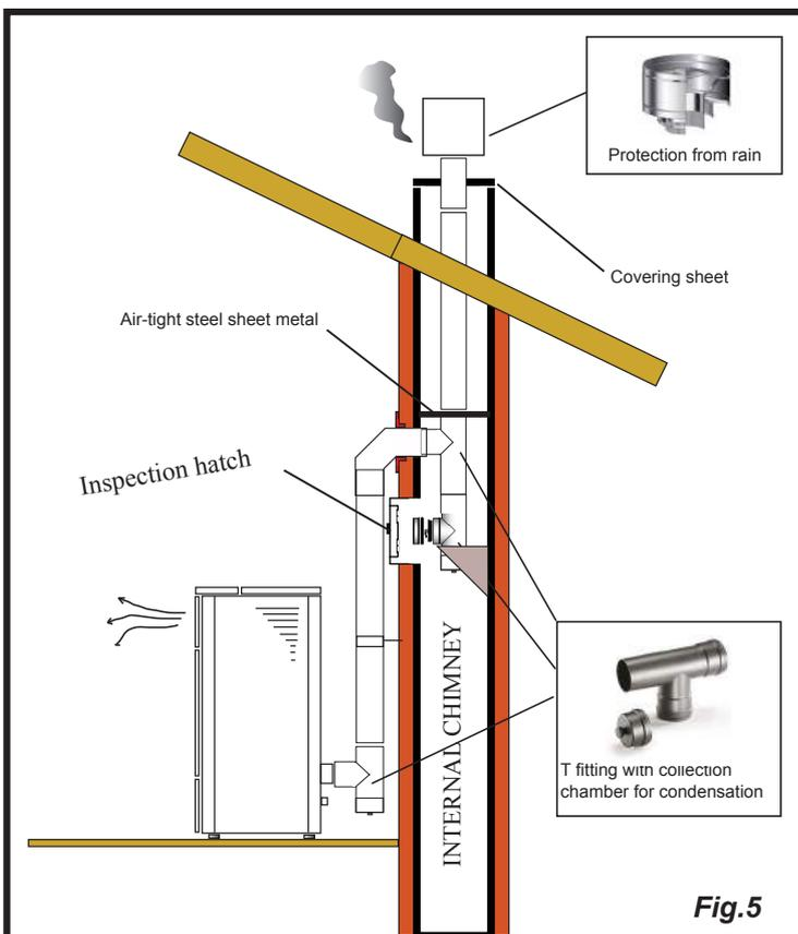
This type of installation (See Fig.5) requires an insulated chimney pot, since the entire smoke conduit is installed inside the building, and the part is located inside a pre-existing chimney pot.
