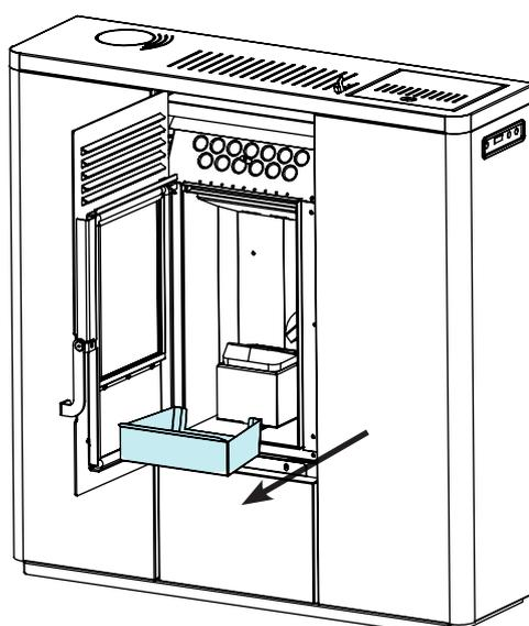
**Removing the flame trap:**
