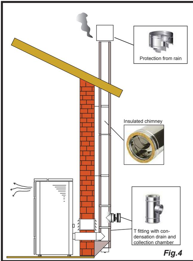
This type of installation (See Fig.4) requires an insulated chimney pot, even if the entire smoke conduit is installed outside the building.
