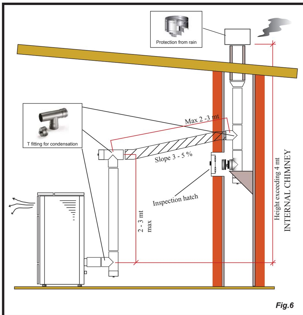
This type of installation (See Fig.6) requires a horizontal section to connect to a pre-existing chimney pot. Respect the slope indicated in figure, in order to reduce the ashes depositing in the horizontal tube. In the lower part of the chimney pot, there is a "T" type fitting installed with inspection cap, in the same way as the chimney pot opening.
