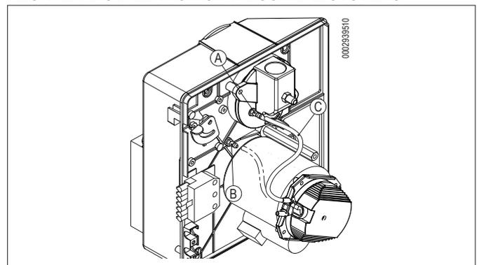
If the air pressure switch measures a value less than the minimum calibration value, remove the tube "C" from the pressure port "A" and connect it to pressure port "B".
