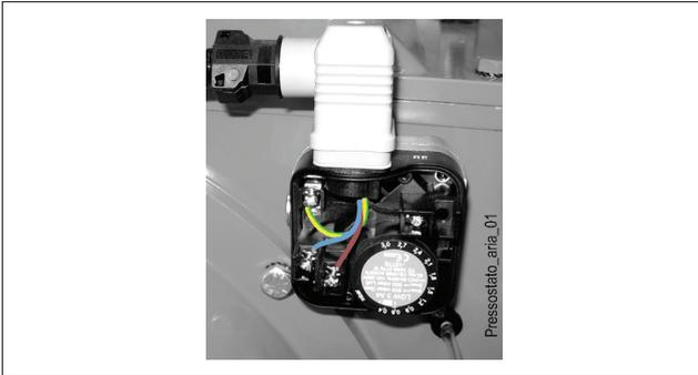
The gas pressure switches (minimum and maximum) prevent the burner from operating when gas pressure is not between the expected range.
