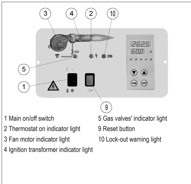
Then passing on to minimum or maximum power through the progressive opening of the gas throttle and the air damper at the same time.
