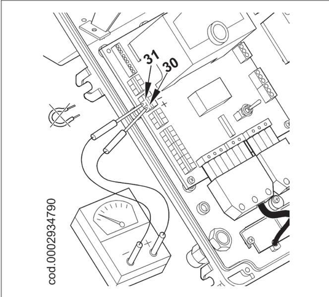
**DIAGRAM FOR REGULATING THE ELECTRODE DISK DISTANCE**
