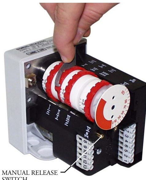
Remove cover to gain access to the adjusting cams. The cams are to be adjusted through the suitable key provided for. Description:
