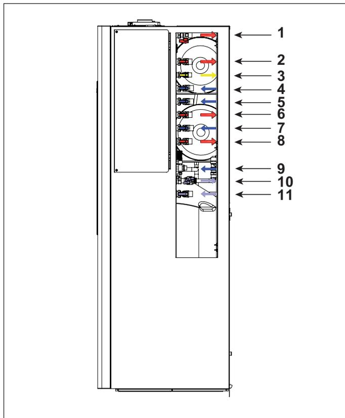
Fig. 7 Schema idraulico Madeira Solar Compact KBS Z
