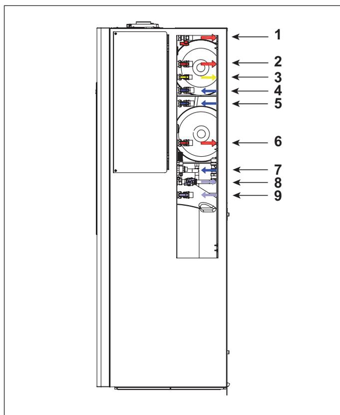
Fig. 6 Schema idraulico Madeira Solar Compact KBS V
