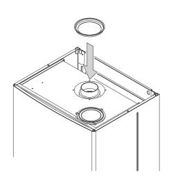
For discharge types C12, use the diaphragm  $\emptyset$  79.0 supplied with the boiler, only when the length of the coaxial duct is less than 1 metre.
