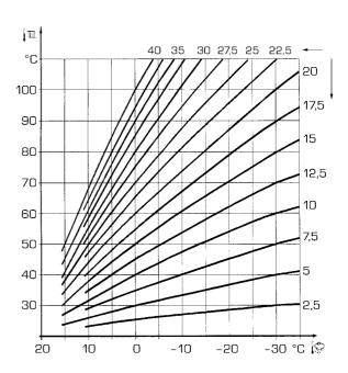
ATTENTION: curves are calculated at an ambient temperature of 20°C. Using the  $\parallel \parallel \parallel$  key on the control panel, the user can change the set ambient by  $\pm$  5°C for which the curve is calculated.
