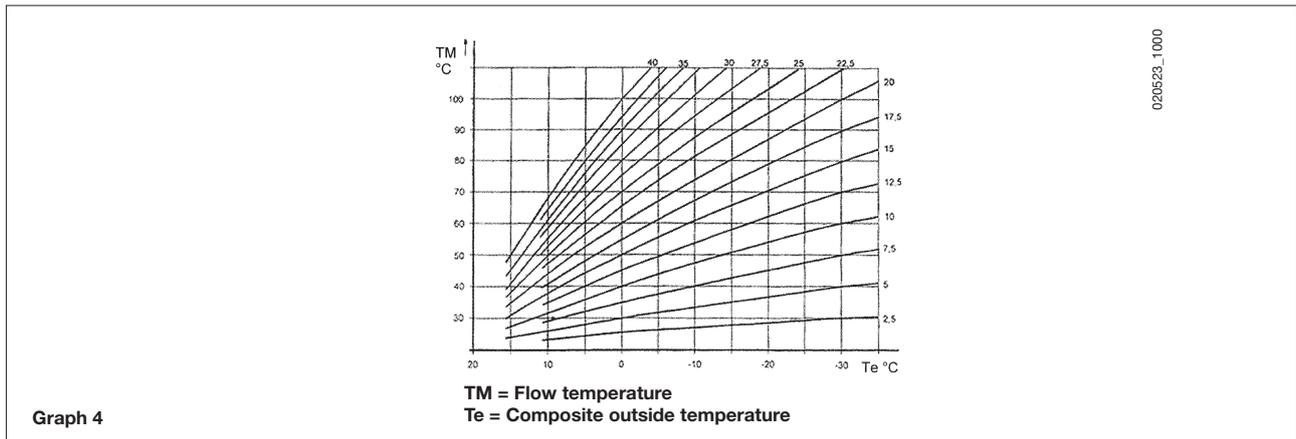
**c) with AGU2.500 device for control of a low temperature system:**
