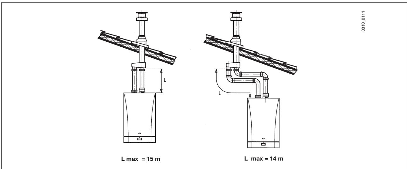
**IMPORTANT:** if fitting a single exhaust flue duct, ensure it is adequately insulated (e.g.: with glass wool) wherever the duct passes through building walls.
