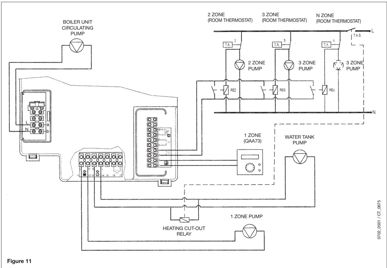
**c) with AGU2.500 device for control of a low temperature system:**
