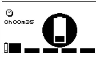
The charging duration is displayed on the screen. As soon as charging is complete, the battery flashes. Disconnect the charger: the stimulator will switch off automatically.
