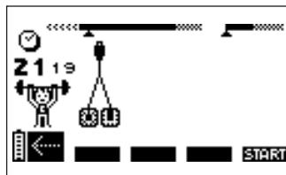
The device emits a tone and alternately displays the pair of electrodes symbol and an arrow pointing towards the channel on which a problem has been detected. In the above example, the stimulator has detected an error on channel 1.
