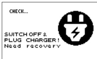
If a battery is very flat, a recovery cycle will start, lasting 2 minutes.
