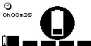
The charging duration is displayed on the screen. As soon as charging is complete, the battery flashes. Disconnect the charger: the stimulator will switch off automatically.
