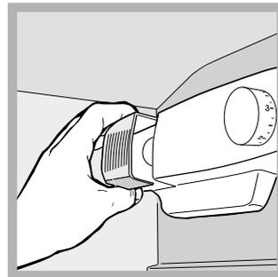
Access the light bulb by removing the cover as indicated in the diagram. Replace it with a similar light bulb within the power range indicated on the cover (15W or 25W).
