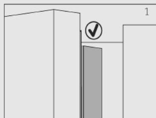
If you try to close the left door and the vertical door beam is unbent (2), you should bend it firstly, otherwise the door beam will hit the fixing shaft or right door. Thus a damage to the door beam or a leak will occur.
