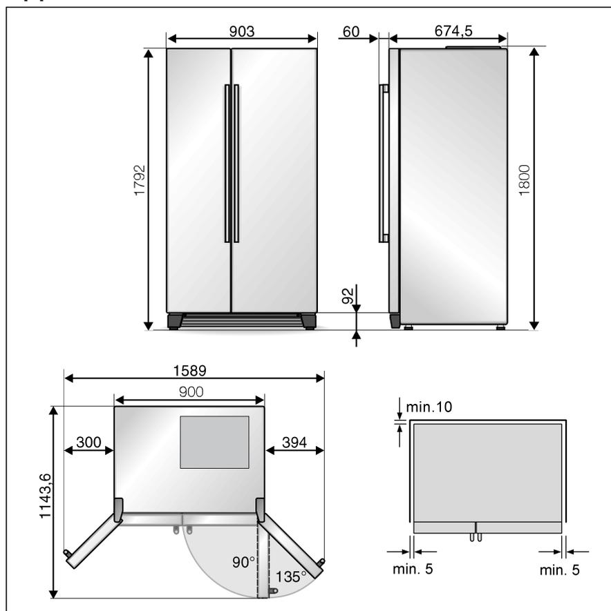
If the depth of the adjacent kitchen equipment is more than 60 cm, observe lateral minimum distances in order to utilise the full door opening angle.
