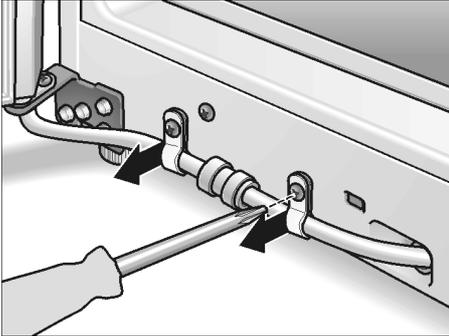
Press the clamping ring in the direction of the arrow and simultaneously pull the hose out of the hose connection.
