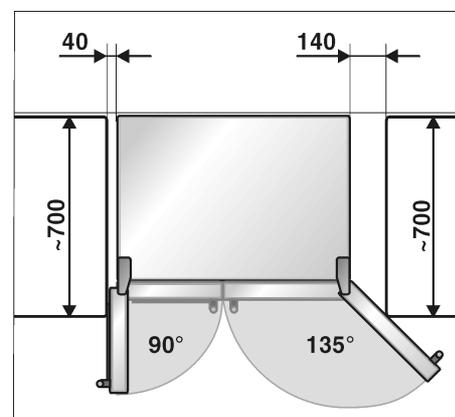
If a panel or cupboard is installed above the appliance, ensure that a gap is left so that the appliance can be pulled out of the recess if required.
