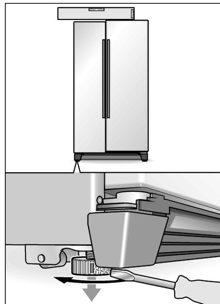
Refrigerator compartment door is deeper:
