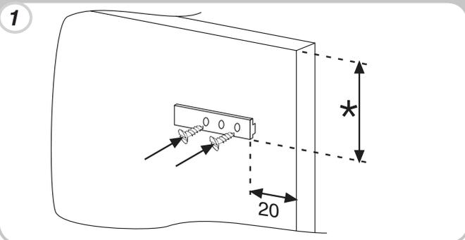
Open the doors of the built-in column and the fridge. Position the built-in loader in the slide, then fit it into the fridge door.
