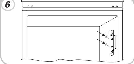
Remove the hole cover plugs, as indicated in the figure.
