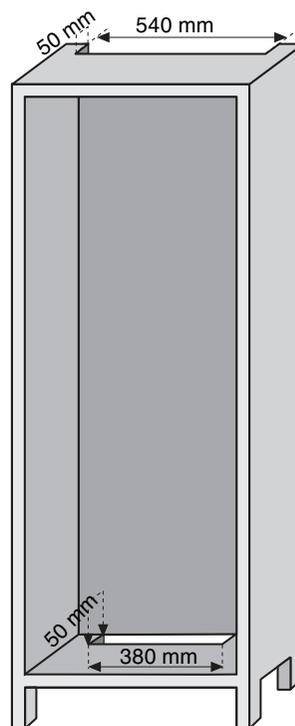
Dimensions of the gap to be left between the column and the ceiling.
