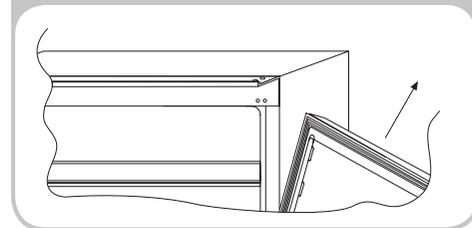
Remove the pin of the bottom right-hand side hinge and remount it on the bottom left-hand side hinge.
