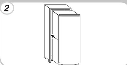
Fasten the bottom part of the appliance with the screws provided.
