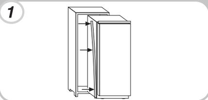
Fasten the top part of the appliance to the cabinet, using the screws provided.
