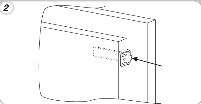
Mark the fixing points for the screws and drill with a bit of a diameter of 2.5.
