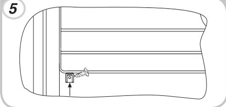
Unscrew the hook positioned on the left-hand side of the freezer compartment.
