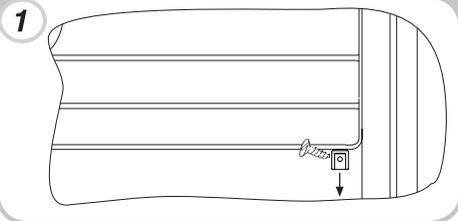
Position the door and hinge first and then screw the latter to the product.
