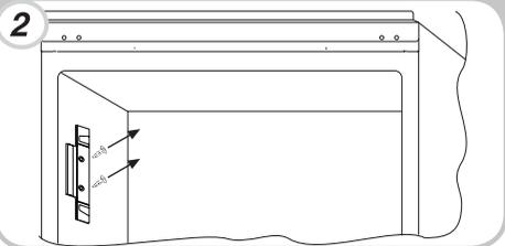
Screw the hook on the right-hand side of the freezer compartment.
