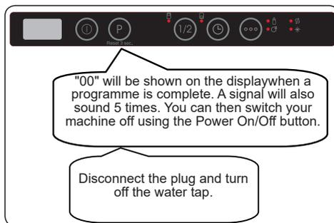
**NOTE:** If any button is not pressed on the ready state, the machine turns off automatically after 15 minutes.
