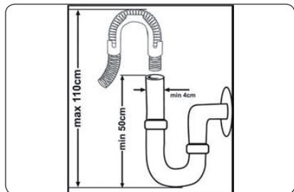
Connect the water drain hose directly to water drain hole or to the sink outlet spigot. This connection should be minimum 50 cm and maximum 110 cm from floor plane.
