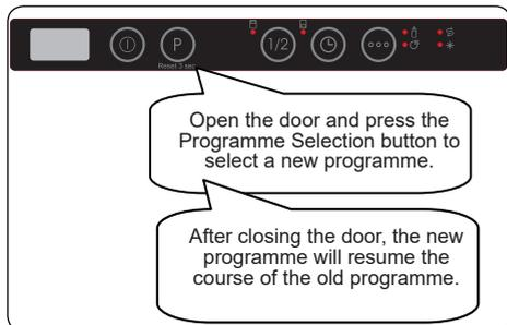
**NOTE:** Open the door slightly at first to stop a programme before it is complete in order to avoid water spillage.
