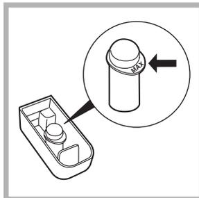
This option is particularly useful for the removal of stubborn stains. Place extra compartment 4 (supplied) into compartment 1. When pouring in the bleach, be careful not to exceed the "max" level marked on the central pivot (see figure).
