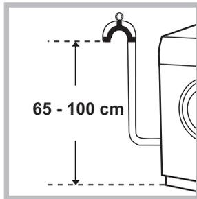
Connect the drain hose, without bending it, to a drainage duct or a wall drain located at a height between 65 and 100 cm from the floor;
