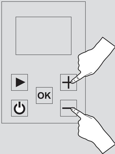
This function is used to lock the keypad, excepting for the On/Off key .
