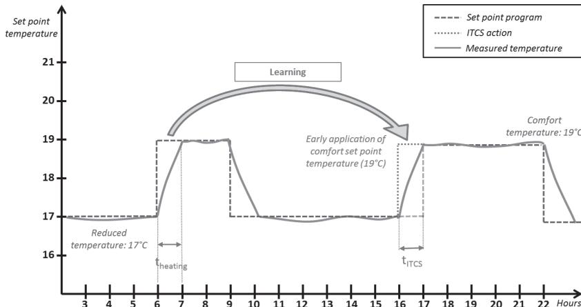
To operate, the ITCS system automatically performs several time and temperature measurements. The objective is to estimate a heating rate for the system. With this value, the system can calculate the heating activation time in advance.
