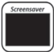
If there is no activity on the keypad for 5 to 10 seconds, a screen saver is displayed. This screen saver could be the value of the measured or zero temperature:
