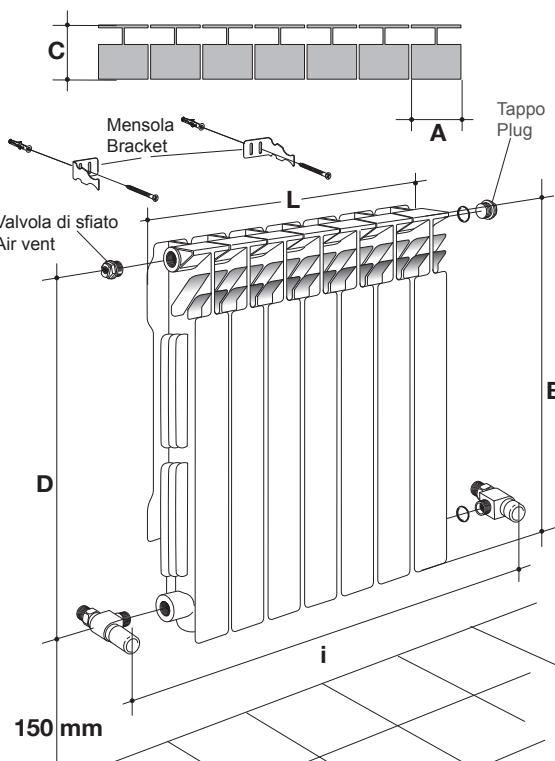
$L = A \times n^{\circ}$  elementi /  $A \times$  no. elements
