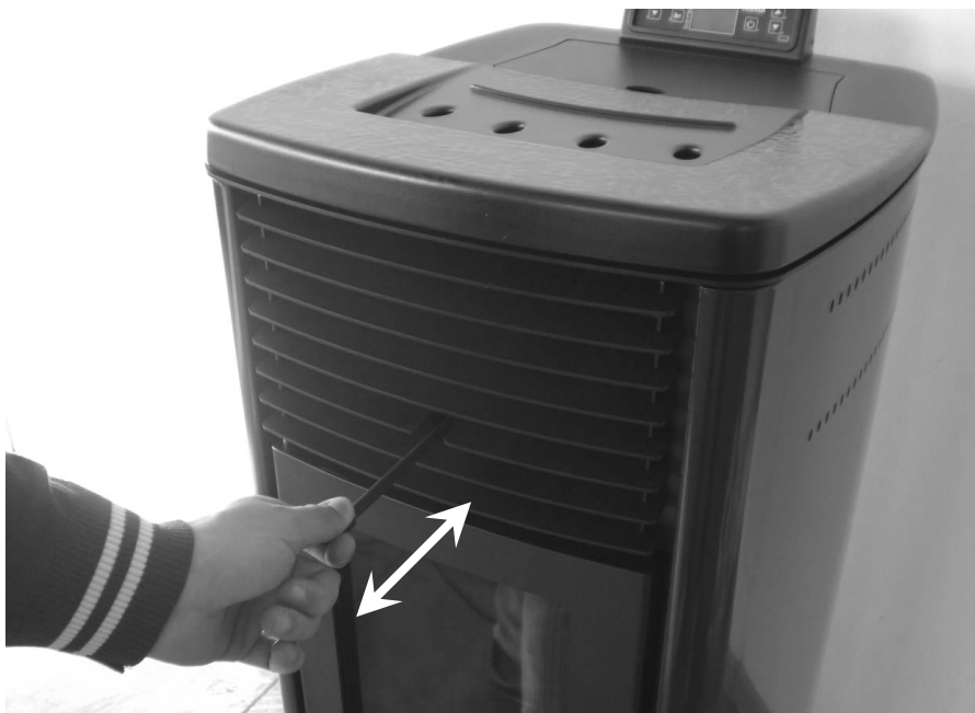
Pull front knob to clean the ventilated hot air tubulars above the combustion chamber. Activate knob only with stove off and cold.
