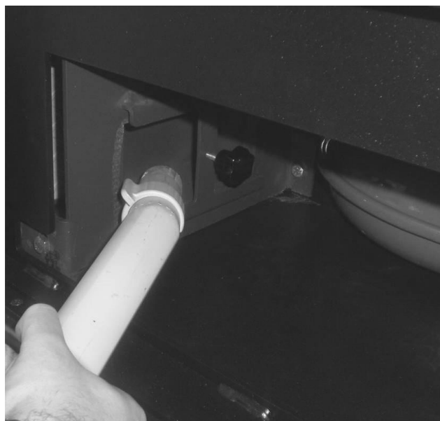
After having unscrewed the hand wheels, extract the lateral plates. Use a suitable suction device to remove internal deposits and then re- close the pipes, making sure that the plates have been fixed well. Reposition the underlying front panel.
