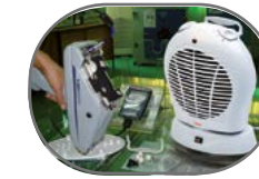
CONTROLLO E SCANSIONE COMPONENTI ROHS / COMPONENTS ROHS CONTROL
