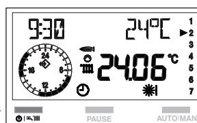
**⚠** To return to the automatic operating mode after a period of manual functioning, you need to press the button AUTO/MAN until the display shows the " ⓘ" symbol.
