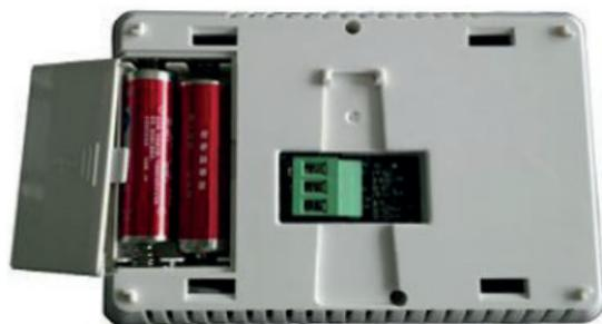
correctly, the thermostat can be applied, taking care to insert the batteries (2 alkaline or zinc / carbon size AA) in the appropriate compartment, respecting
